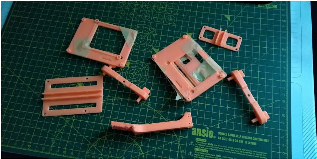
Figure 21: 3D printed mounting plates
