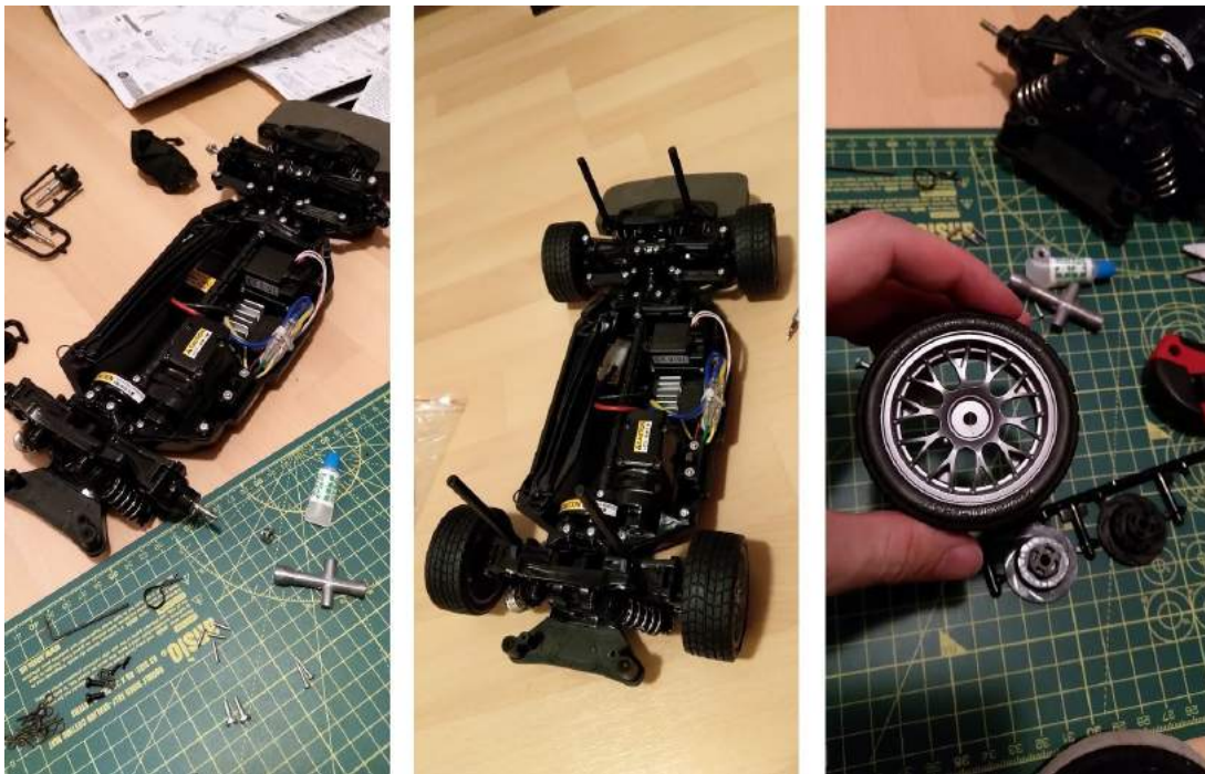
Figure 19: TT-02 RTR Assembly
