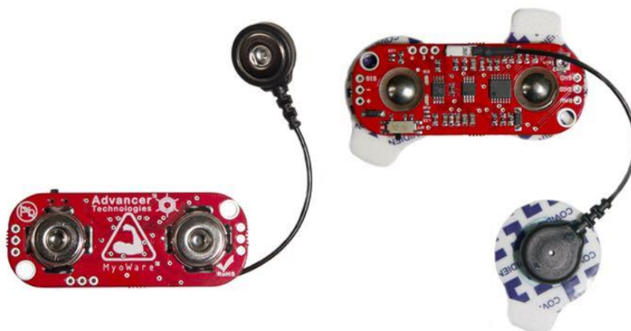
Slika 45. Muscle Sensor (AT-04-001) [47]
