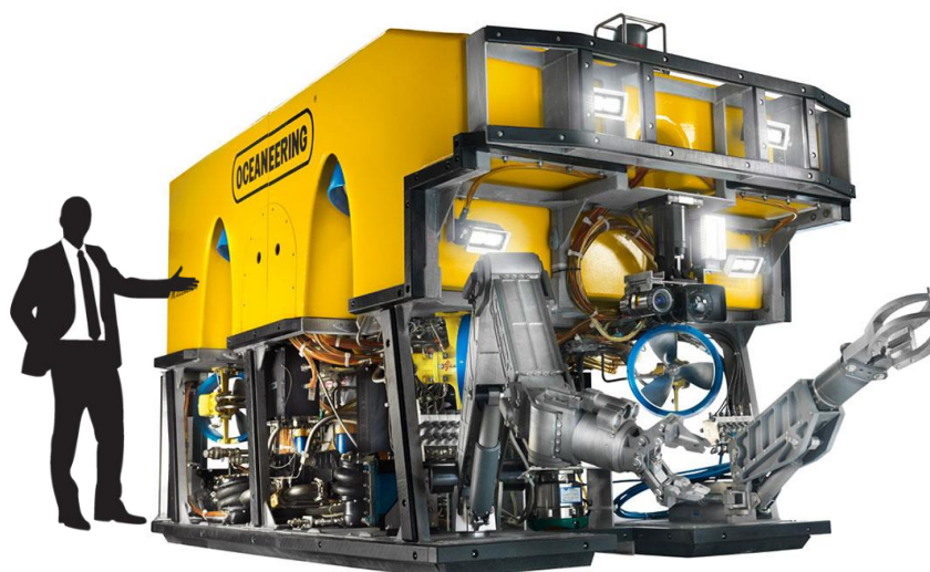
Slika 2.6 Oceanering Millennium Plus Work class ROV (165kW)
