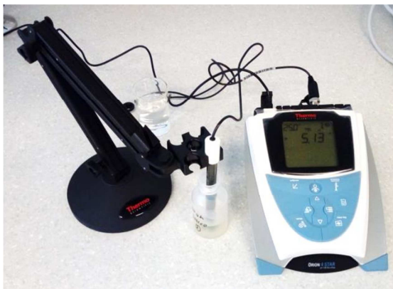
Slika 2.2. pH-metar Orion 4 STAR Thermo Scientific.
