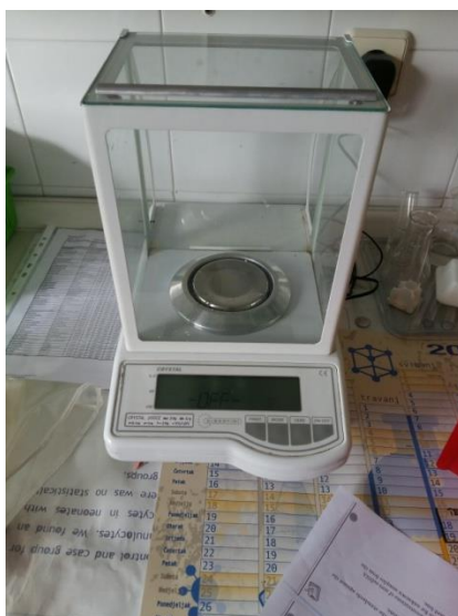
Slika 10. Elektronska vaga s četiri decimalne (Gibertini CRYSTAL 200 CE Magnetic Compensation Analytical Balance, Novate Milanese, Italy).
