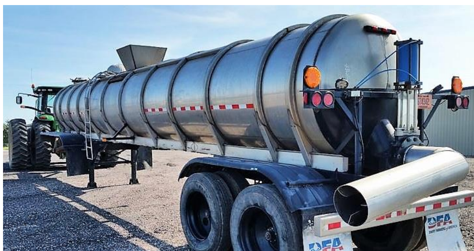
Slika 4. Spremnik za gnojovku (Izvor: https://www.fastline.com/farm-equipment/listing-detail/1985-brenner-stainless-steel-manure-semi-tank-phils-pumping-fab-inc-chilton-wisconsin/9aca64d7-dfdd-4729-805c-d739e794e925.aspx )
