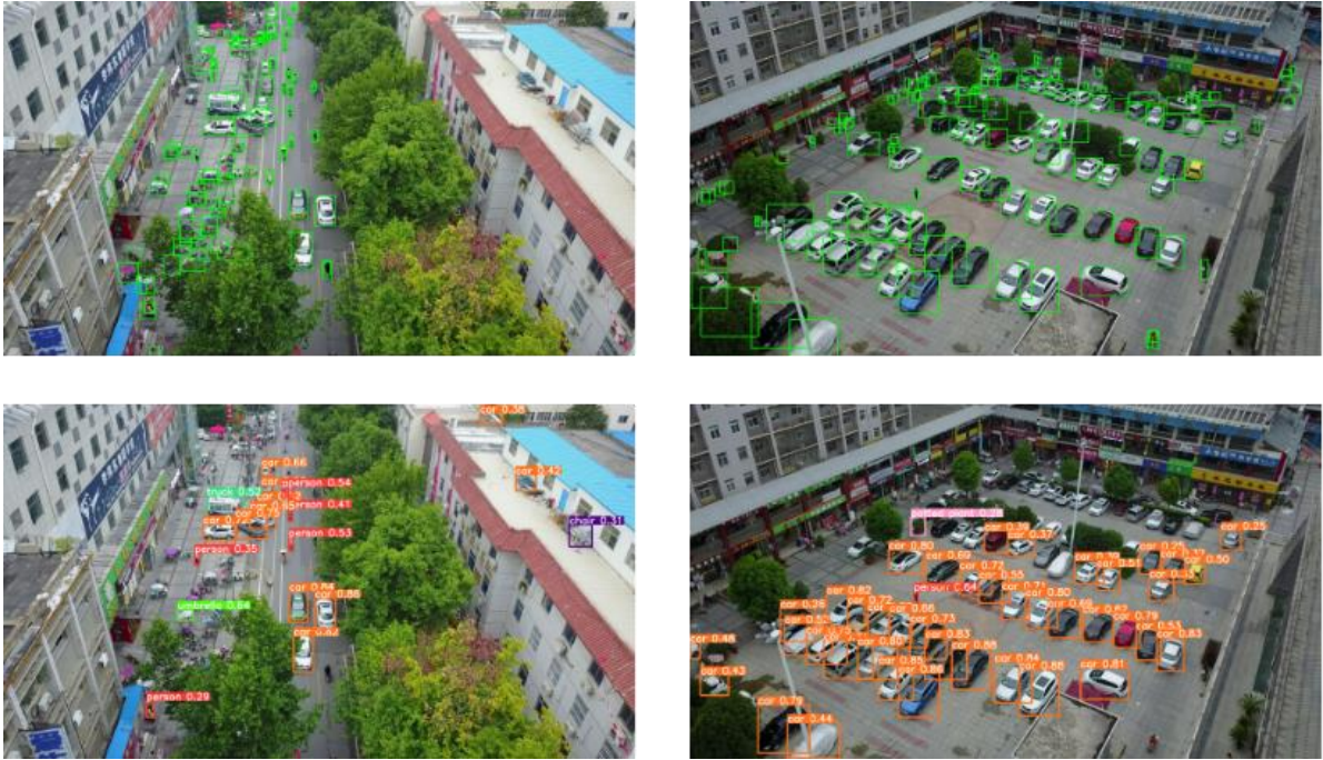
Figure 1.3.1.1 Comparison between ground truth and YOLOv8x predictions (pre-trained on MS COCO) on arbitrarily selected pictures from the VisDroneDET-2019 validation set.
