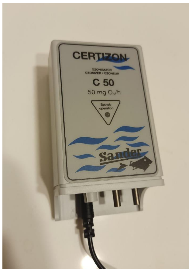
Figure 8. Ozone generator used in the experiment (source: M. Prečanica).
