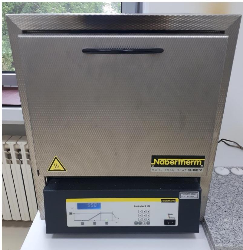
Slika 7: Nabertherm B 170 mufolna peć
