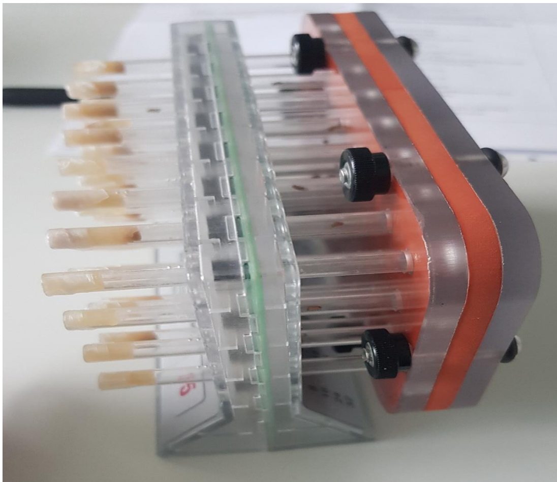
Figure 4. The DAMS monitor and dispenser. The photo shows how the tubes with individual flies are attached to the monitor and the dispenser.
