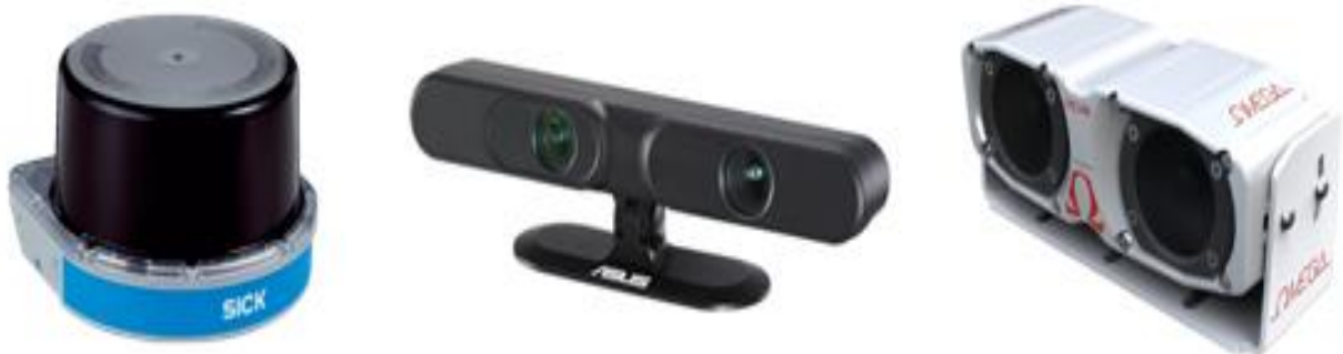
Slika 2.1 LIDAR (Sick), RGB-D kamera (Asus Xtion Pro) i stereo kamera (Omega). (Slike preuzete sa stranice: https://www.sick.com/at/en/detection-and-ranging-solutions/3d-lidar-sensors/mrs1000/c/g387152 , https://www.asus.com/3D-Sensor/Xtion_PRO/ , https://arcure.net/omega-stereo-camera-for-indoor-outdoor-applications )
