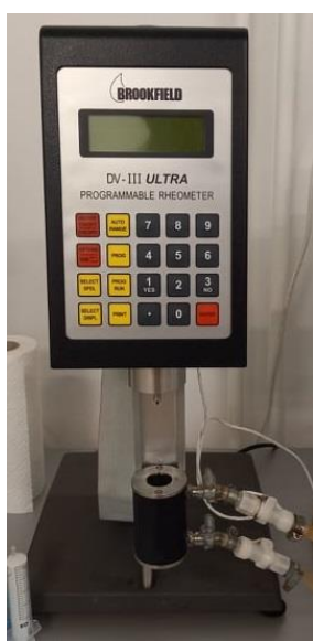
Slika 11. Reometar DV-III Ultra Rheometer by AMETEK Brookfield
