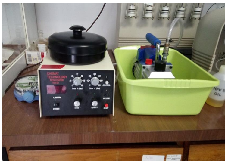
Slika 12. Spin coater , Chemat Technology.
