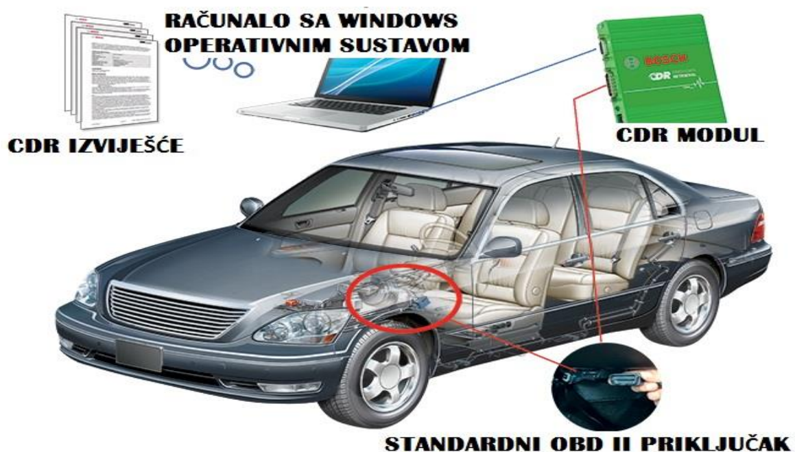
Slika 8. Metoda Direct To Link
