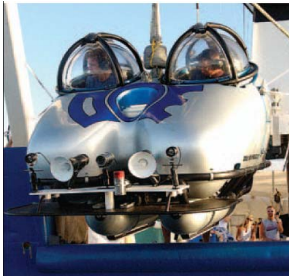
Slika 2. Dual Deep Worker Submersible
