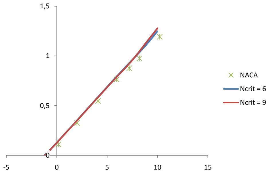
Slika 2.4.2: Usporedba rezultata  $c_l(\alpha)$  za  $Re = 2 \times 10^6$
