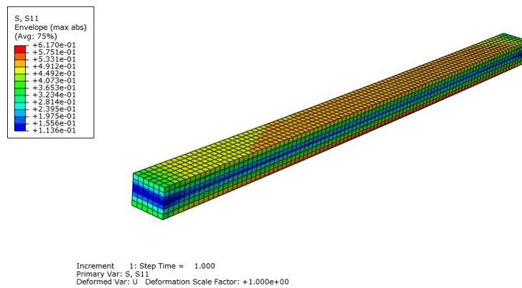
Slika 5.16: Naprezanje u baterijama u osi  $X$  [MPa]
