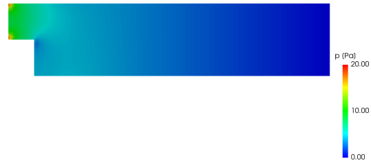
Figure 5.1.21: Backward facing step IBM pressure field visualization, laminar simulation
