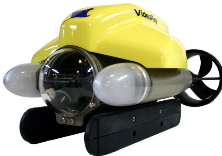
Slika 2.9 VideoRay PRO4 Observation class ROV (5Kg)
