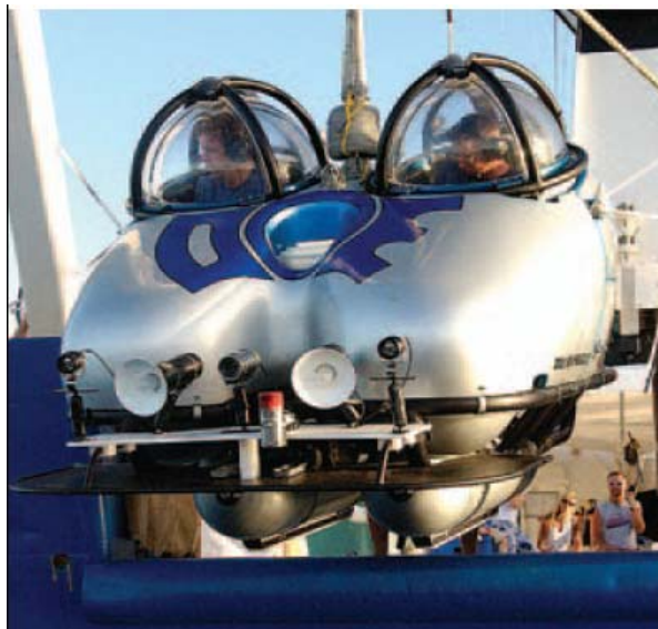
Slika 2. Dual Deep Worker Submersible
