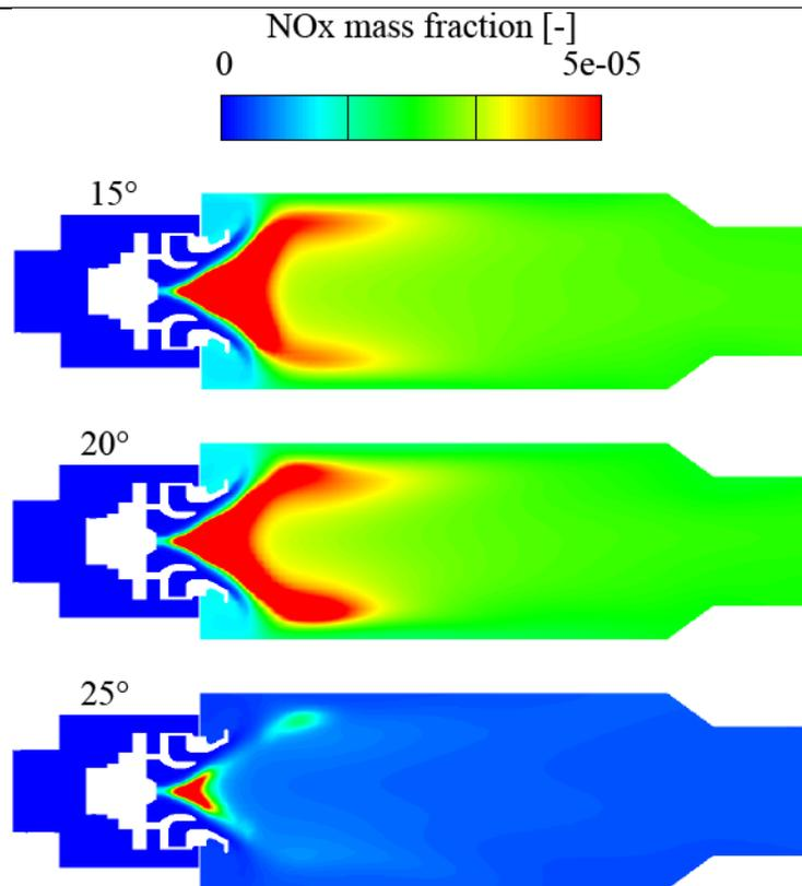
Figure 22 NOx distribution for different spray angles
