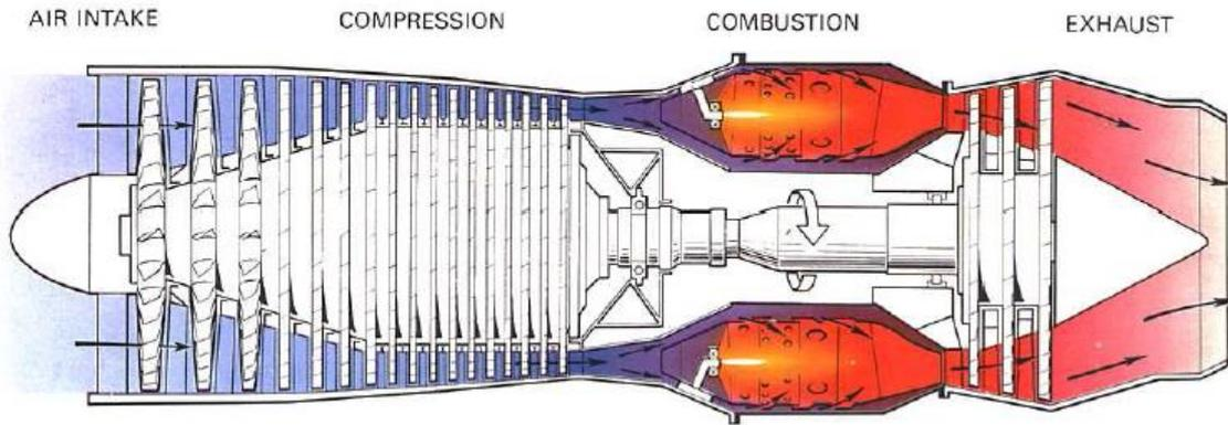
**Figure 2 Schematic of processes within the jet engine [3]**
