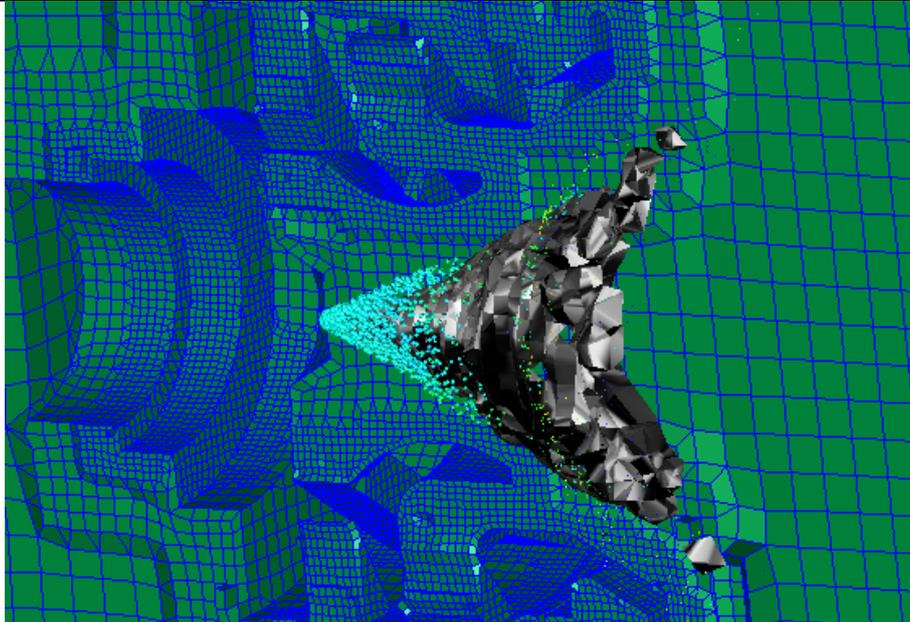
**Figure 24** Isosurface of evaporated fuel with spray angle  $20^\circ$
