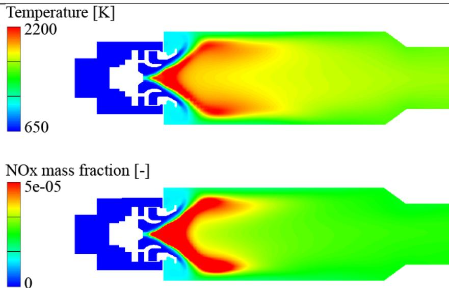
**Figure 26** Temperature (up) and NO<sub>x</sub> (down) distribution at quasi stationary state
