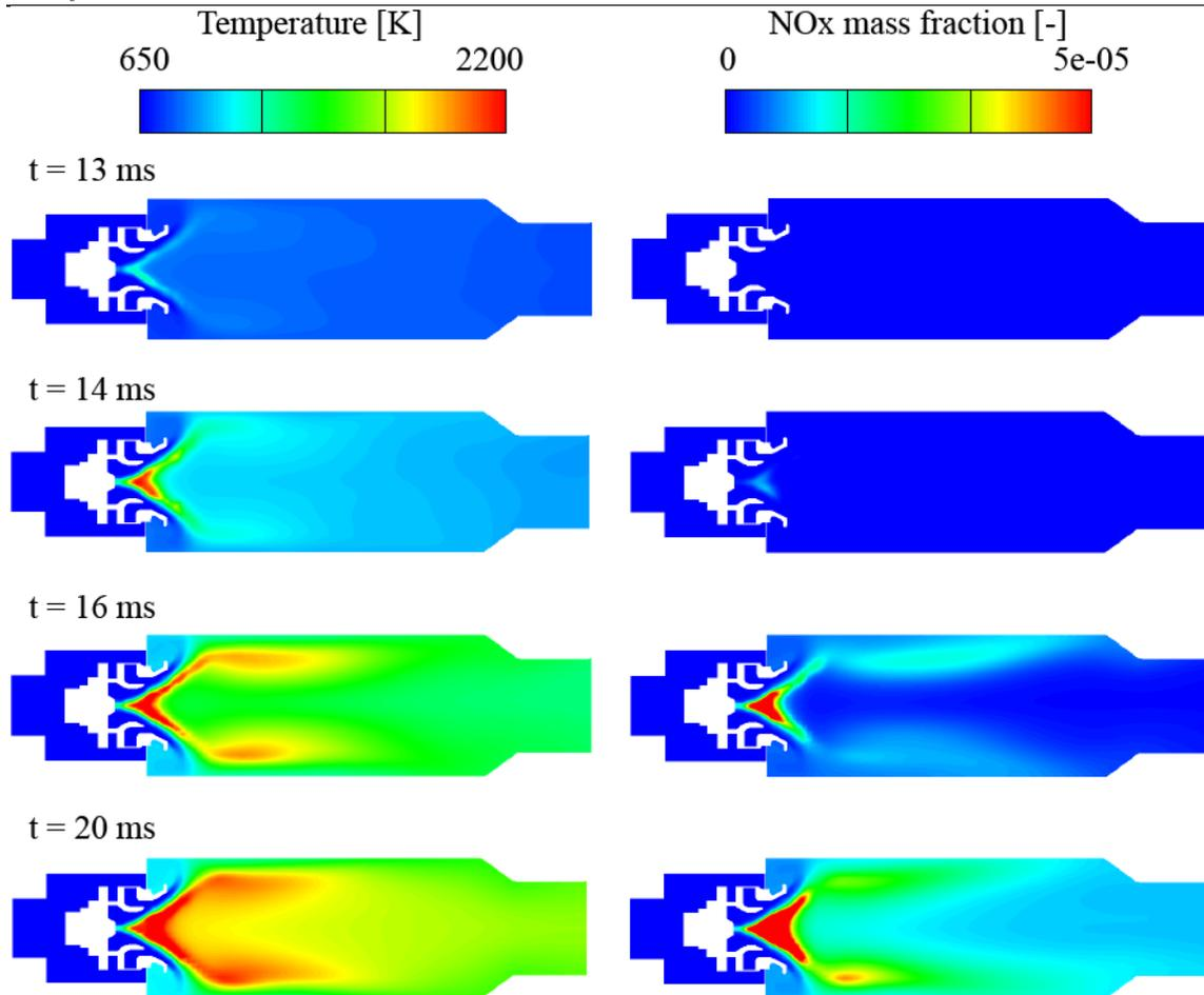
**Figure 25** Temperature and NO<sub>x</sub> distribution through combustion chamber
