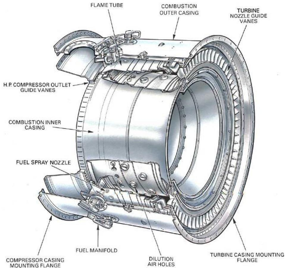
**Figure 8 Annular combustion chamber [3]**
