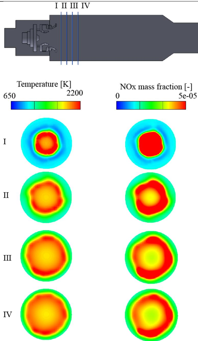
**Figure 27** Temperature (left) and NO<sub>x</sub> (right) distribution at different locations in the streamwise direction
