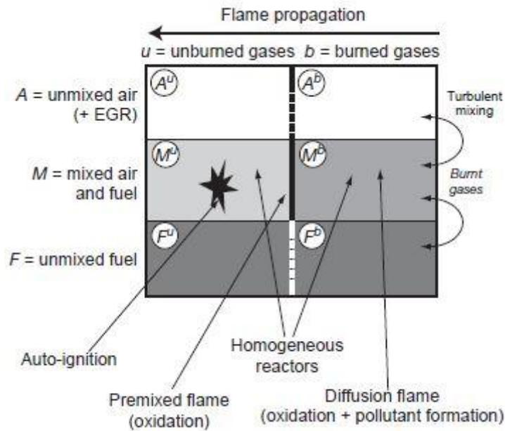
**Figure 9** Schematic of the ECFM-3Z model computational cell [22]
