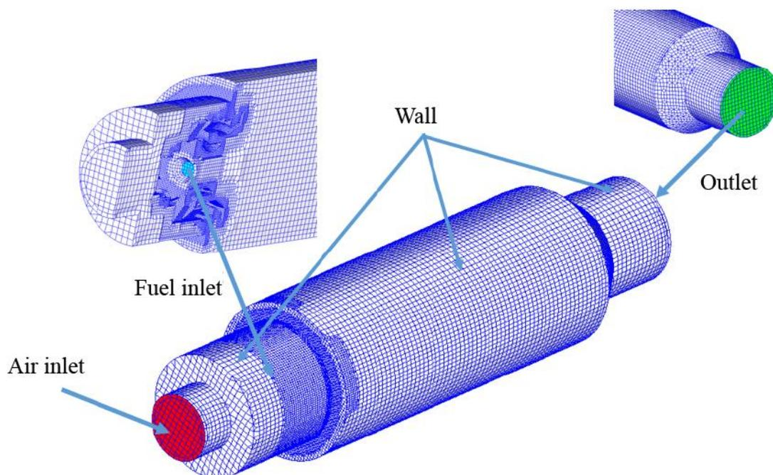
Figure 13 Rough mesh with selections for boundary conditions
