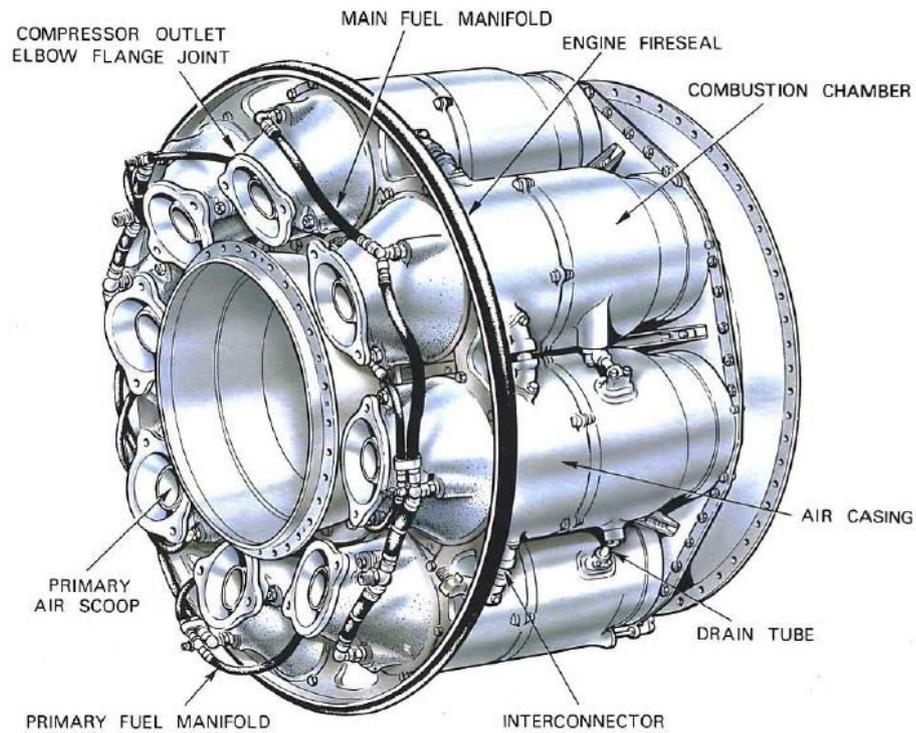
**Figure 6 Multiple combustion chamber [3]**
