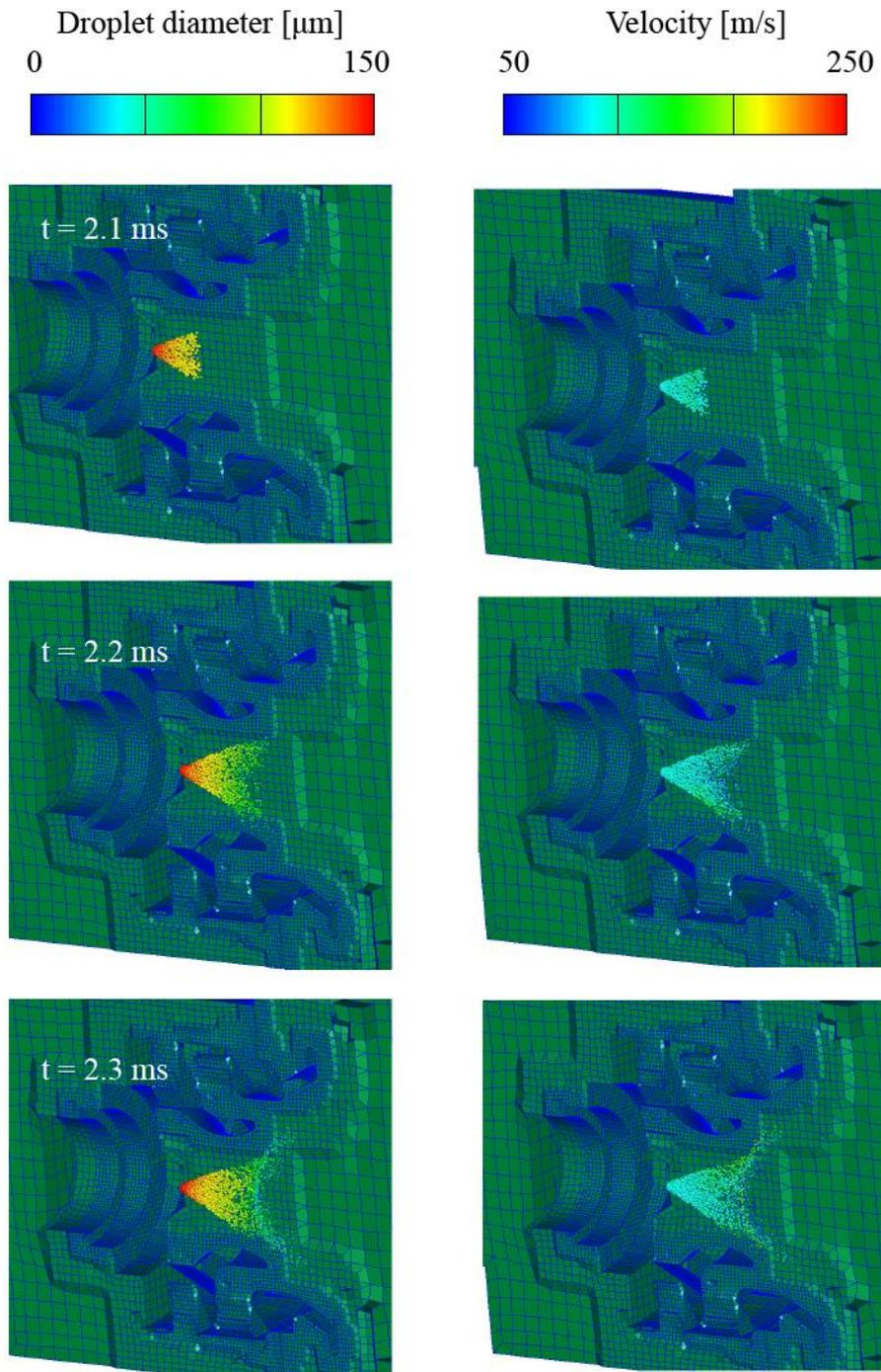
Figure 23 Spray formation with spray angle  $20^\circ$
