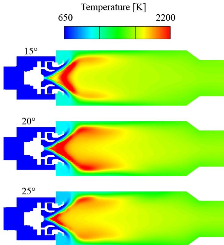
**Figure 21** Temperature distribution for different spray angles
