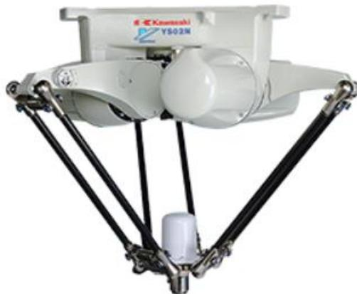
Slika 6. Delta robot *Kawasaki Robot YF002N*
