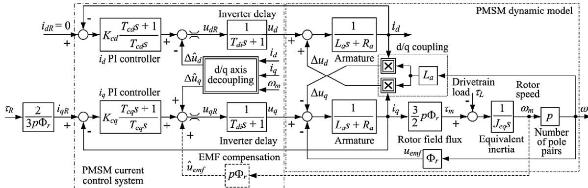
Slika 11. Dinamički model PMSM motora [10]
