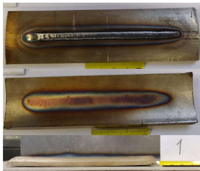
Slika 15. Uzorak 1 ( $I = 75 \text{ A}$ ,  $U = 12,5 \text{ V}$ )
