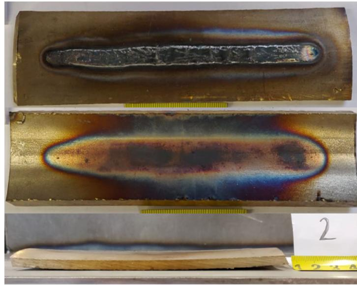
Slika 16. Uzorak 2 ( $I = 100 \text{ A}$ ,  $U = 13,2 \text{ V}$ )
