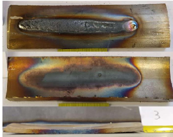
Slika 17. Uzorak 3 ( $I = 125 \text{ A}$ ,  $U = 14 \text{ V}$ )
