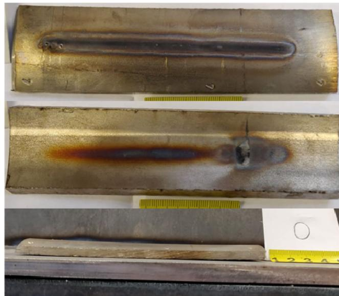
Slika 14. Uzorak 0 ( $I = 50 \text{ A}$ ,  $U = 12,2 \text{ V}$ )
