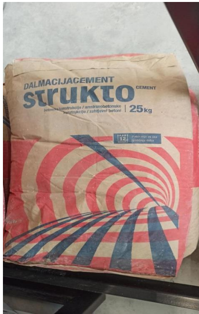
Slika 32 Cement CEM II/B-M (S-LL) 42,5N
