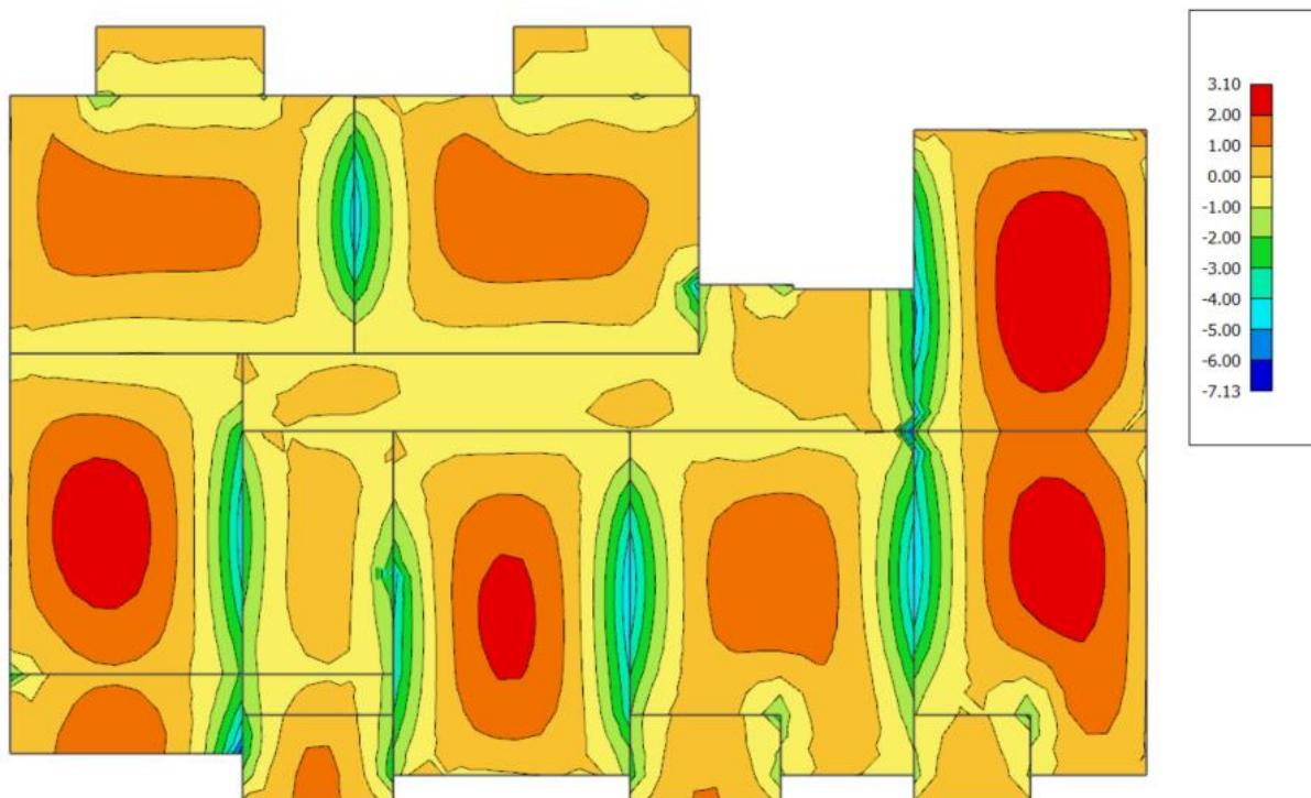
Slika 4.7. Armatura u ploči  $A_{s,x-x}$  ( $\text{cm}^2/\text{m}$ ) za GSN
