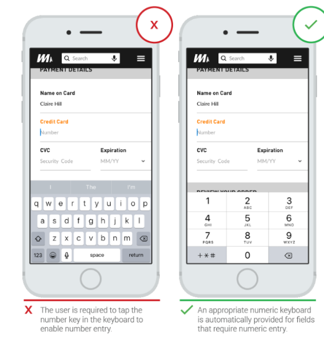
Figure 18. Use masked input and right keyboard rule (source: https://uxplanet.org/designing-more-efficient-forms-structure-inputs-labels-and-actions-e3a47007114f )
