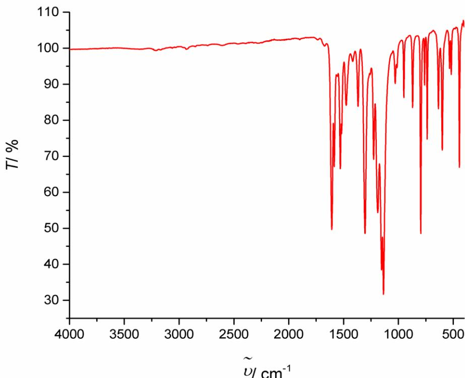
**Slika D11.** IR spektar  $[\text{Cu}(\text{tfac})_2]$
