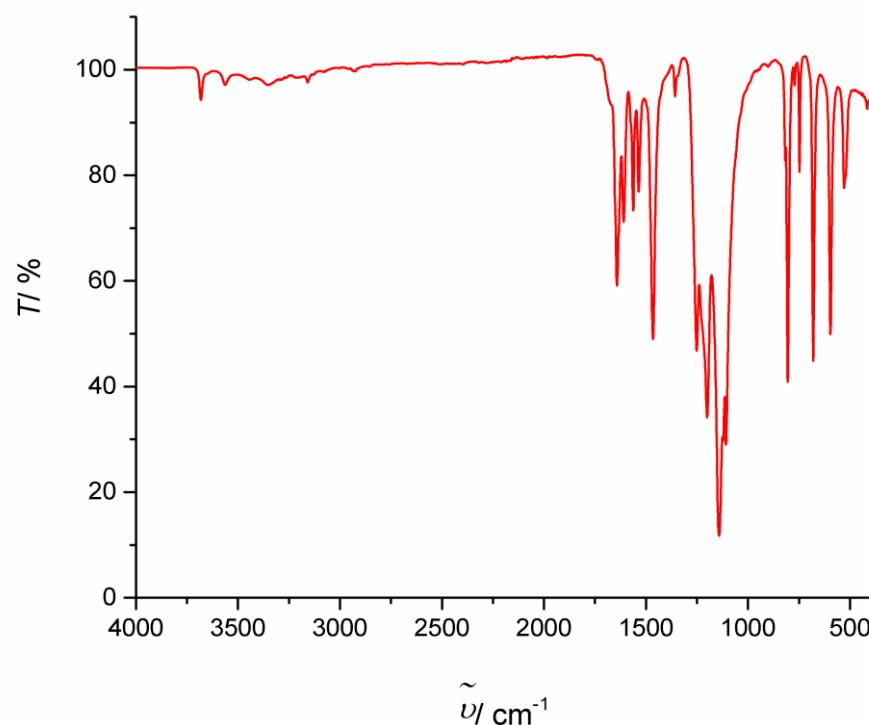
**Slika D12.** IR spektar polaznog spoja  $[\text{Cu}(\text{hfac})_2(\text{H}_2\text{O})_2]$  (**1**)
