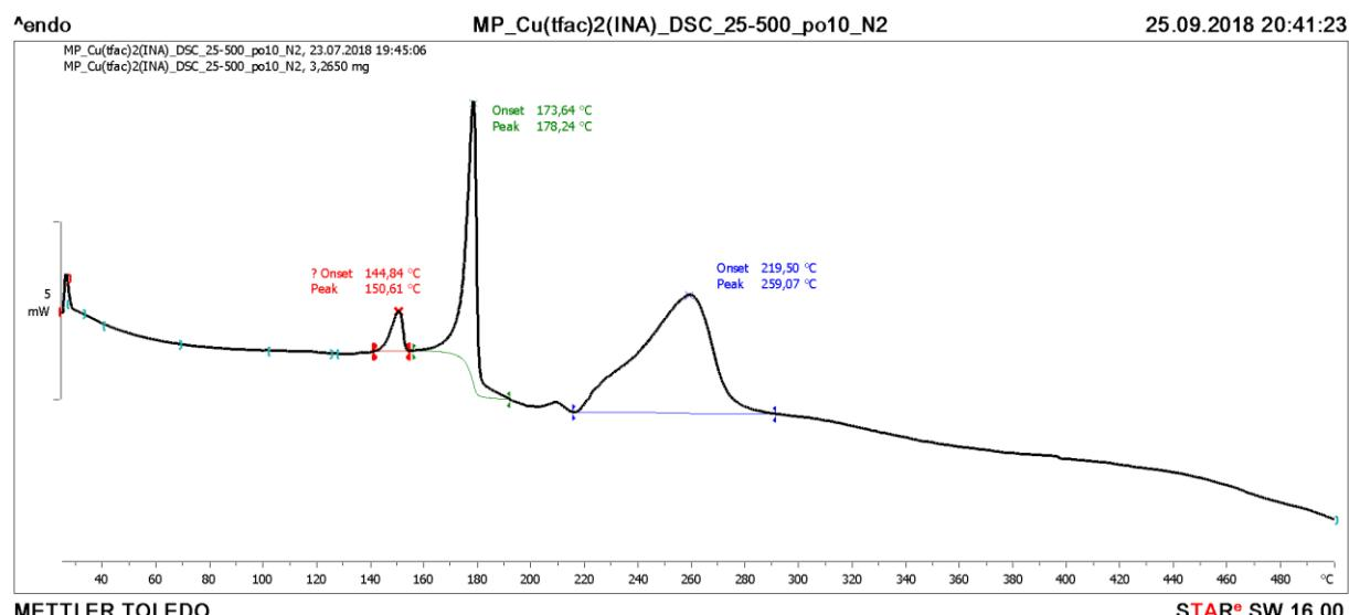
**Slika D30.** DSC krivulja spoja  $[\text{Cu}(\text{tfac})_2(\text{isn})]$  (**2c**)
