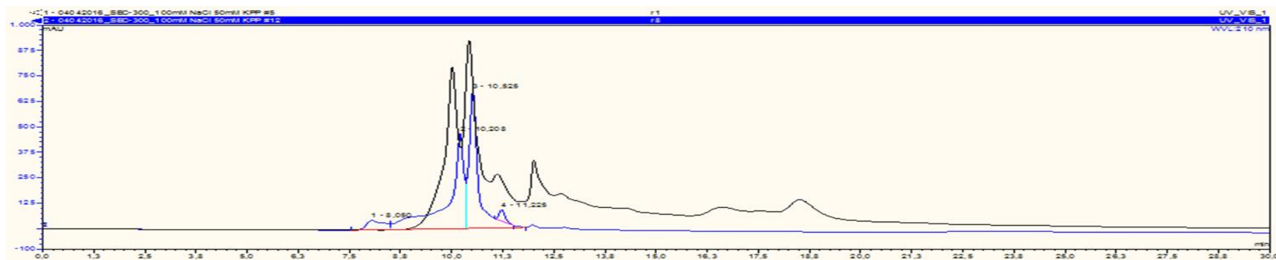
Figure 12. SEC chromatogram of 10 mL lignin solution + laccase. The reference material, lignin solution itself, is shown in black.
