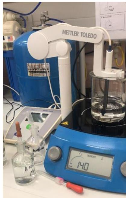
Slika 6 pH metar Seven Easy (Mettler Toledo)
