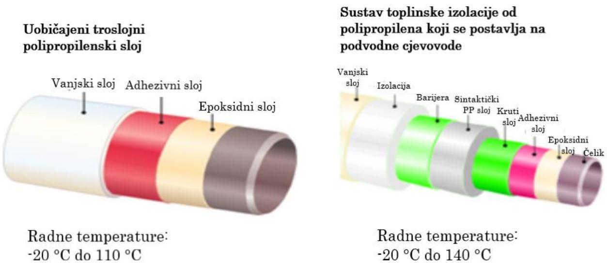
**Slika 4-4.** Sustavi polipropilenske zaštite od polipropilena (Turner, NACE, 2011)
