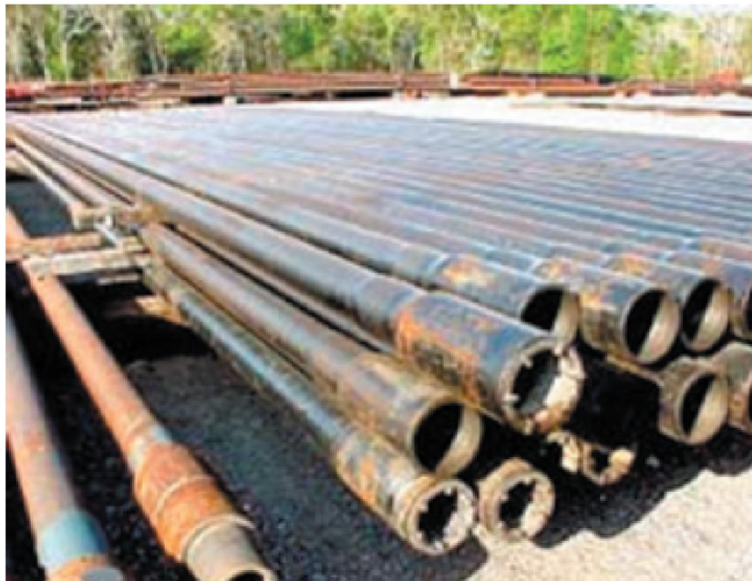
Slika 3-1. Bušaće šipke ( https://en.wikipedia.org/wiki/Drill_pipe#/media/File:Drill_pipe.jpg )
