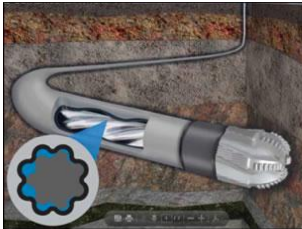
Figure 6-1. Schematic figure of a PDM ( www.laser-ndt.com )
