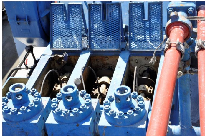
Figure 4-6. 3 cylinder mud pump ( Aydin, 2015)
