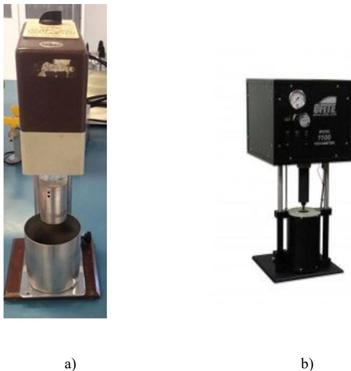
Slika 5-5. Viskozimetar OFITE model 800 korišten u radu a), i Model 1100 Viscometer b) (OFI Testing Equipment, 2018 (d))
