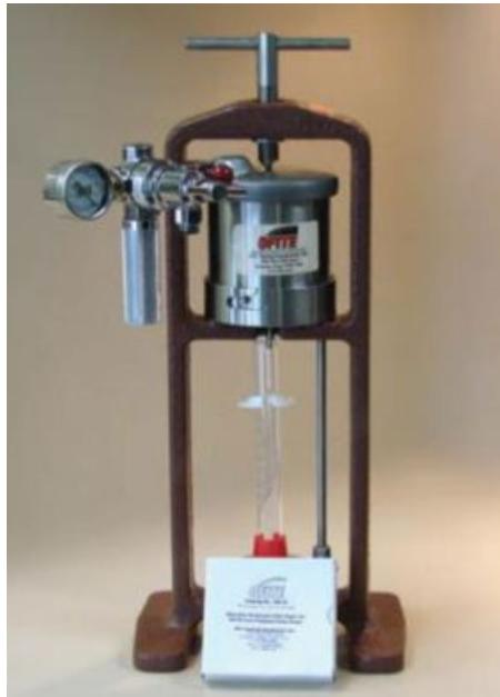
Slika 5-10. API filter preša (OFI Testing Equipment, 2018 (e))
