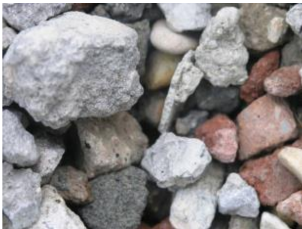
Slika 4-10: Reciklirani agregat (ECO-SANDWICH, 2015)
