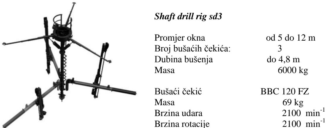
Slika 6-4. Bušaća platforma shaft drill rig sd3 (Deilmann-Haniel Mining Systems, 2016)
