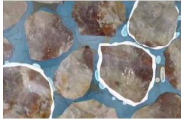
Figure 6-3 Dense CO 2 (g) migrating upwards (light blue bubbles) dissolving and reacting with the grains of the rock, leading to precipitation of minerals on the grain boundaries (white) (CO 2 GeoNet, 2007) ( http://online.fliphtml5.com/iomp/mtiw/#p=1 )
