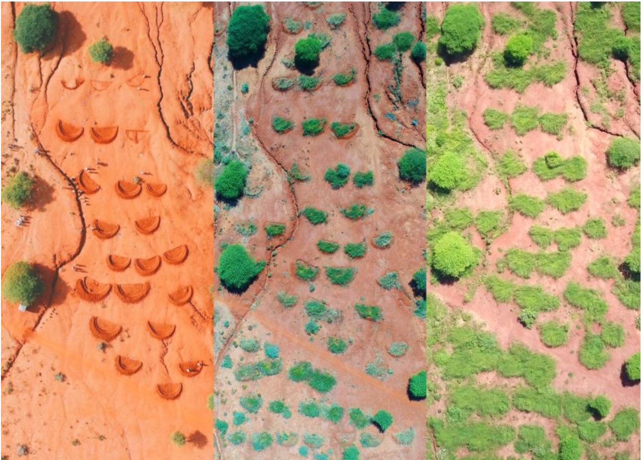
Image 25 A composite aerial image from 2018 to 2020, showing the stages of a greening project in Pemamoto, Tanzania. The halfmoon shaped “bunds” are dug out by humans and then left to collect water and enable autonomous greening of the area.
