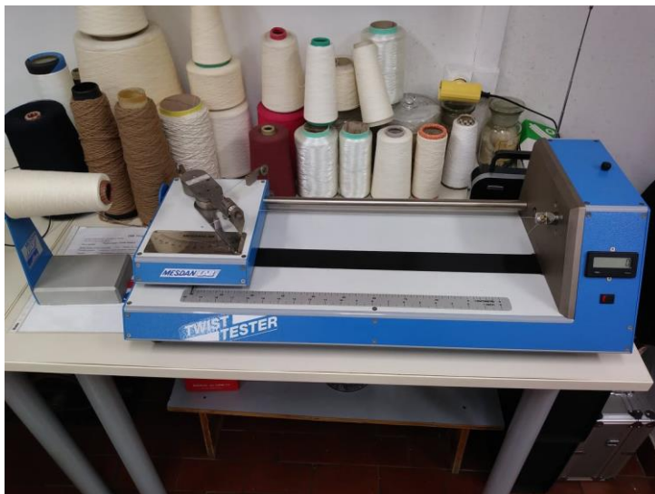
Sl. 20. Torziometar, Twist –T, Mesdan Lab
