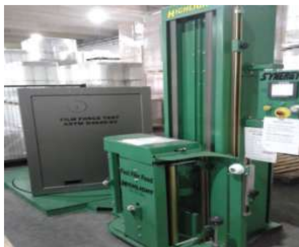
4.13 Highlight's Synergy 4 Test Wrapper [25]
