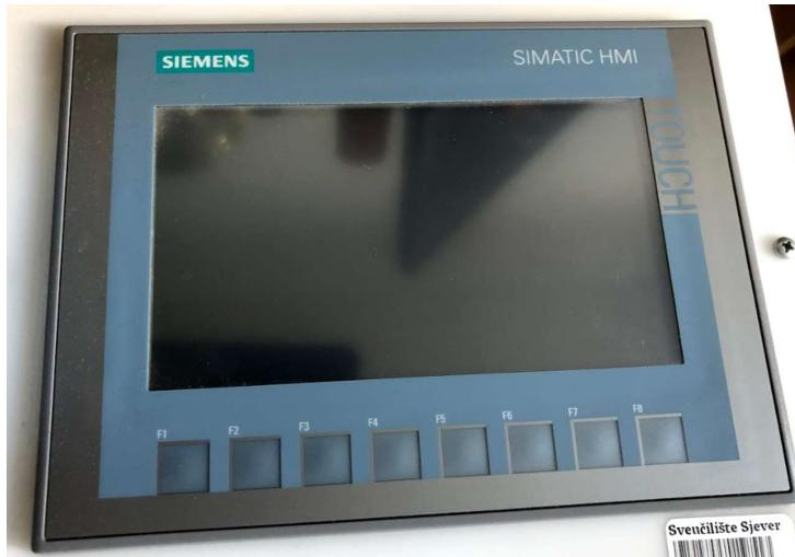
Slika 4. 2 Korišten HMI panel KTP700 Basic PN
