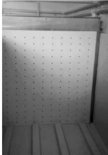
Slika 4. Perforirana pregrada ( www.seafish.org/media/Publications/SR720_Medium-scale-system.pdf )
