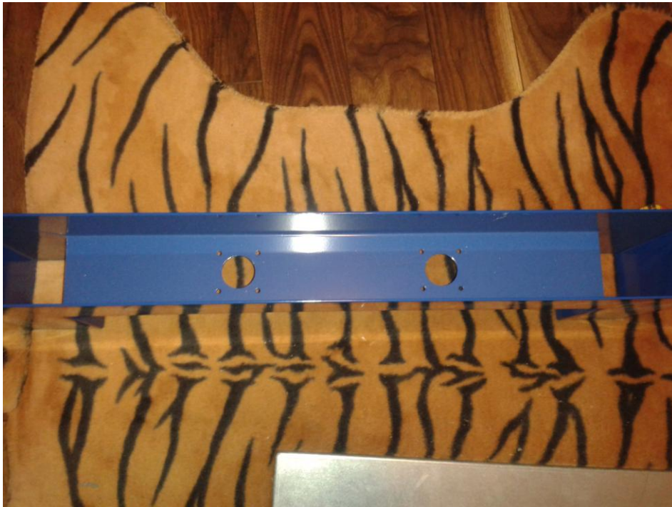
Figure 2.10. Inside of the base construction showing holes for stepper motors
