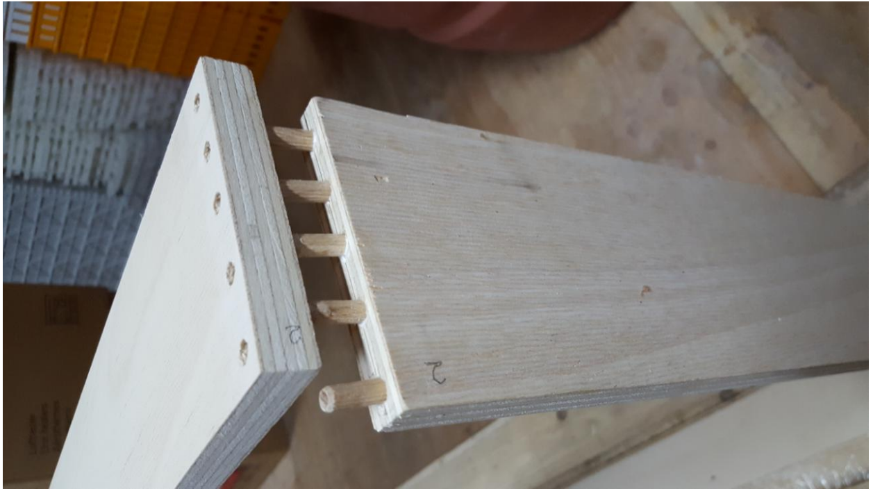
Figure 2.4. Adding the other side of the frame to get one corner piece
