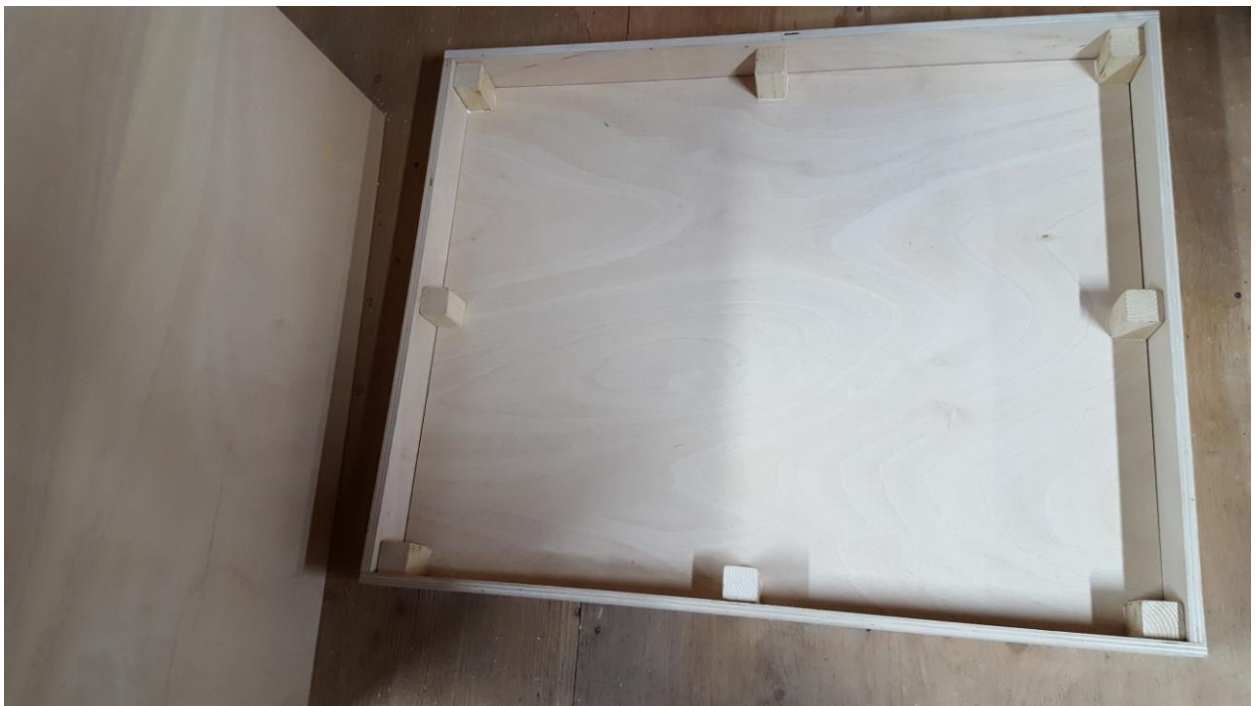
Figure 2.6. Wooden support blocks distributed along the inside frame
