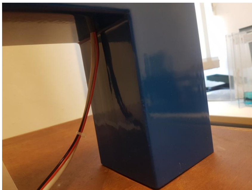
Figure 3.5. Hole for wires from actuator and solenoid
